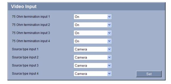
You can activate the 75 Ohm terminating resistance for each video input of the VideoJet X40 SN. The terminating resistance must be deactivated for the video signal to be looped through. Every video input is closed at the time of delivery.
